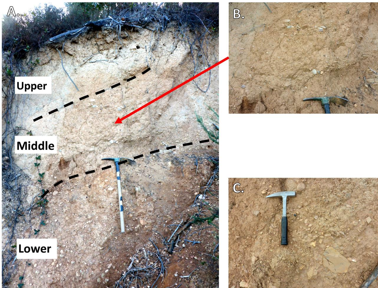
FIGURE 9: A. general view of sidewall of Landslide 8, showing three layers. Charcoal was scattered in the middle and lower layers. The pick is 90 cm long. B. The middle layer is interpreted to be of fluvial origin – note the imbrication of small stones. C. The chaotic lower layer, containing abundant angular stones, is interpreted to be either an old landslide deposit or a colluvial deposit formed by freeze-thaw processes.
