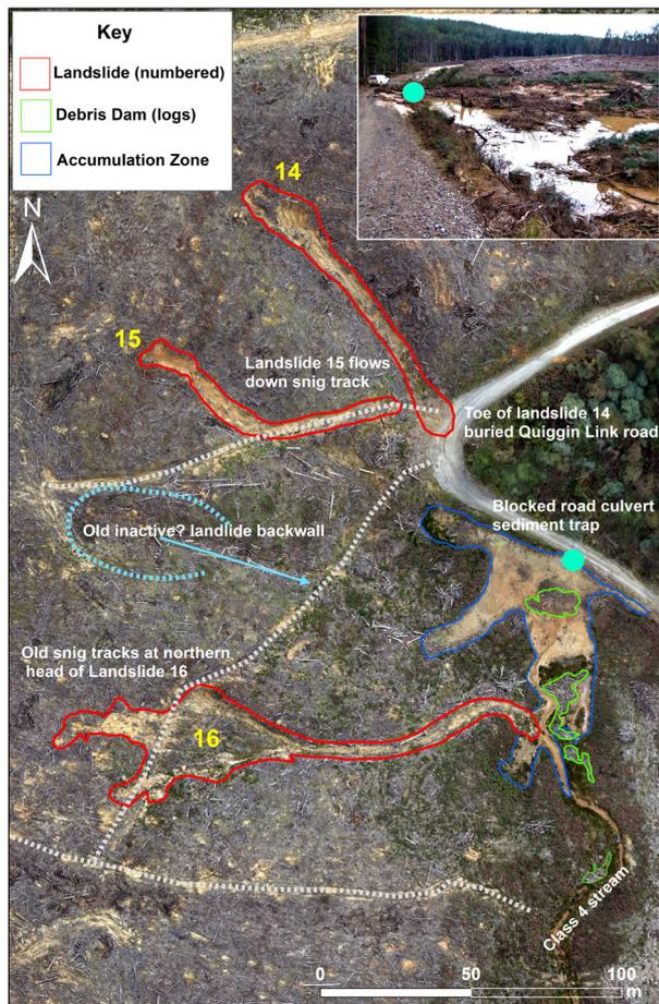
FIGURE 7: Influence of roads, snig tracks (timber extraction tracks) and blocked culverts (green dot in main image and inset image) on landslide initiation and debris accumulation.
