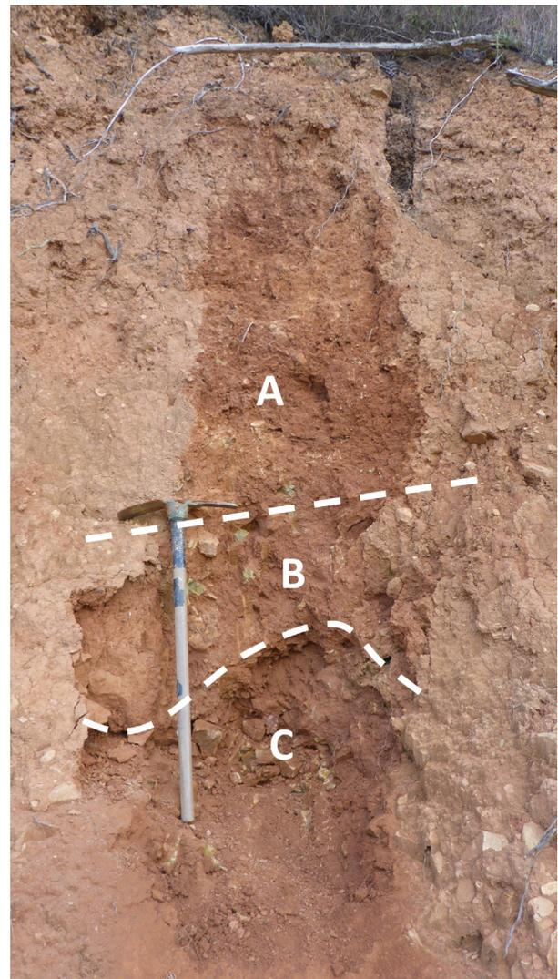
FIGURE 8: Landslide 6, backwall. Three layers are evident: a 1.3 m layer of gravelly silty clay (A), overlying a 30–50 cm deep layer of stony silty clay containing scattered charcoal fragments (B) dated 14.94 cal ka BP, overlying a very stony silty clay deposit (C).
