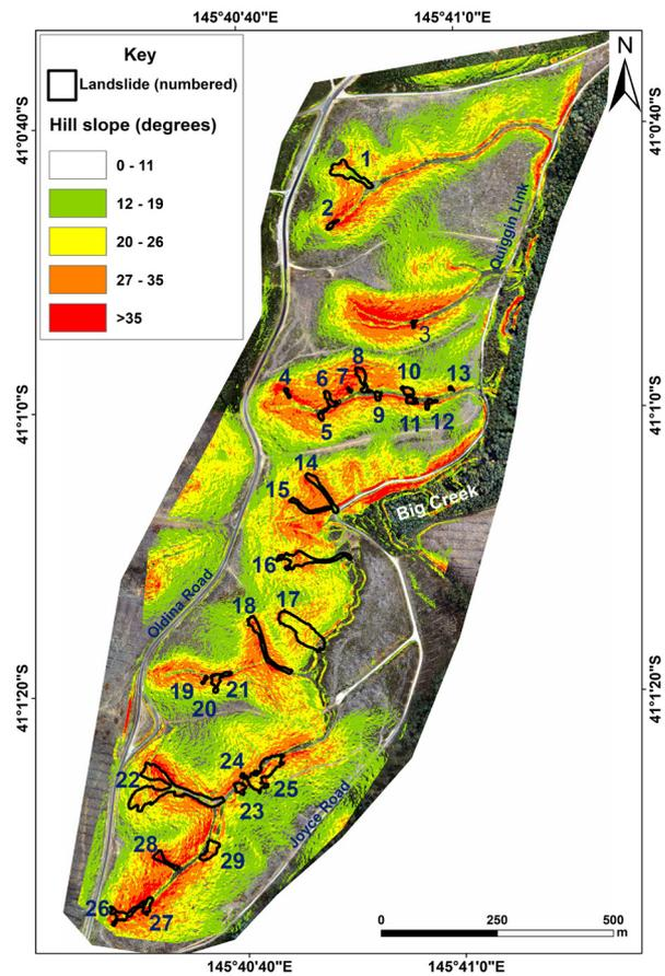
FIGURE 4: Slope map of the study site showing the relationship between the landslides and slopes >26°.
