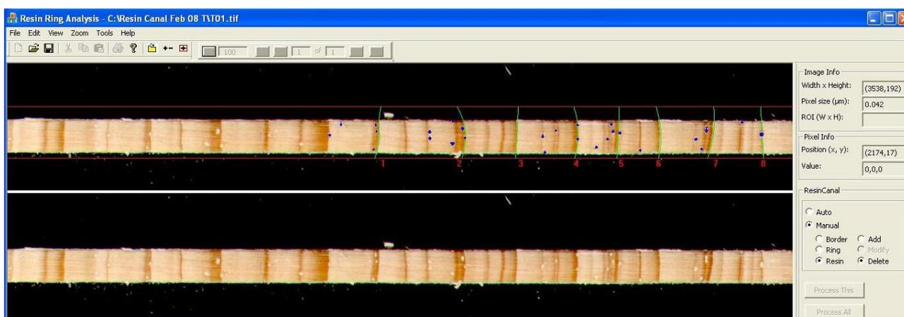
FIGURE 2: A view of the IDL imaging routine used to obtain resin canal information on the 2 mm wide polished transverse surface of a strip from Tangoio Forest. Annual growth rings are marked on the top strip, and show the frequent occurrence of false growth rings at Tangoio Forest. Resin canals are identified and their area and brightness measured.
