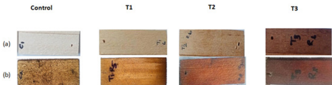
FIGURE 5: Samples before (a) and after (b) fungus infestation
