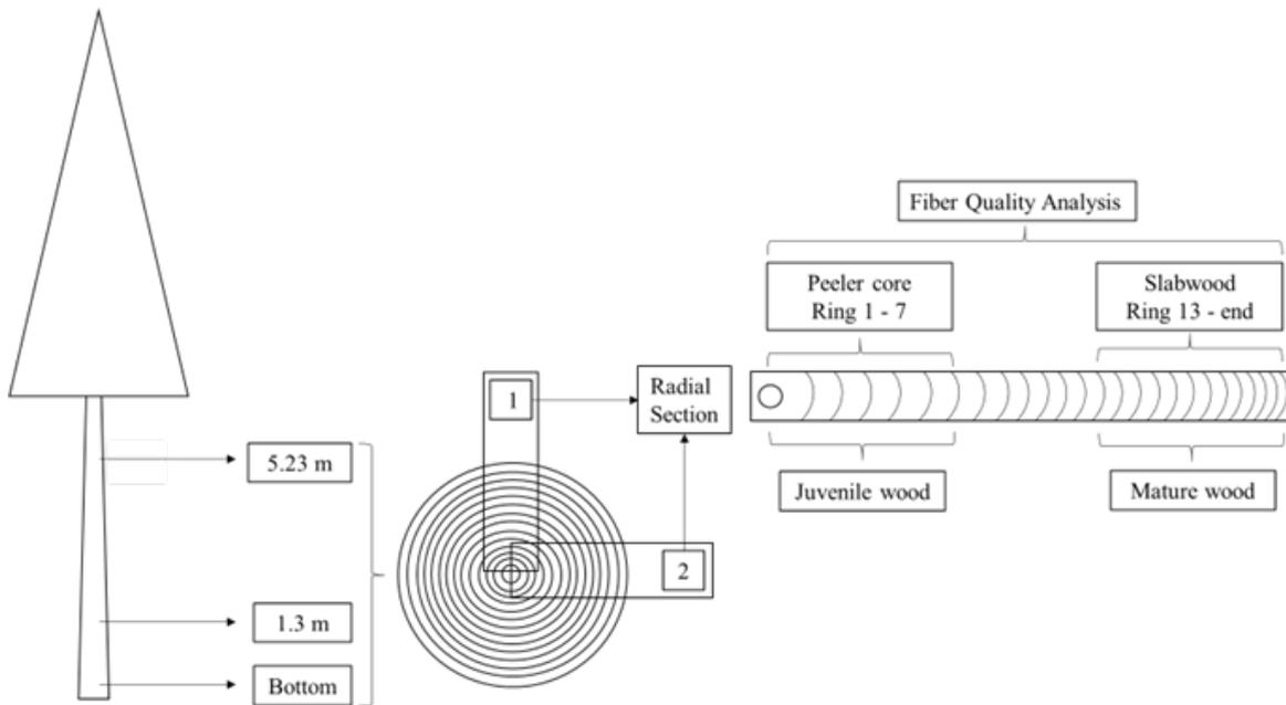
FIGURE 3: Illustration of the sampling process to obtain the wood sections per disc, for fibre quality analysis.
