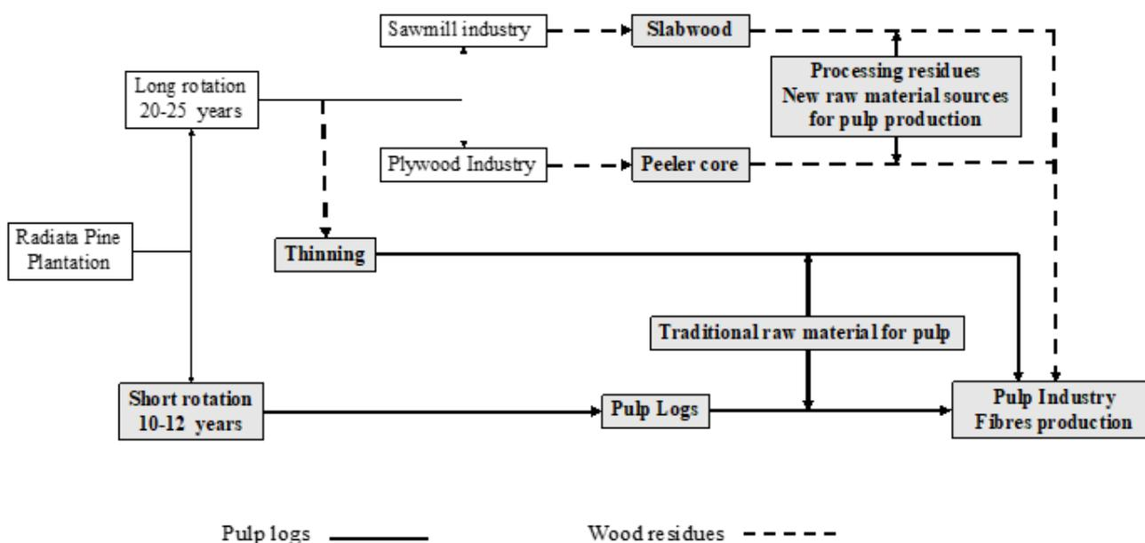
FIGURE 1: Diagram of the raw material sources (pulp logs and residues) to produce pulp from *P. radiata* in Chile.
