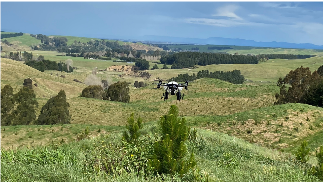
FIGURE 6: Field trial with UASS preparing to spot spray individual trees. (Photo courtesy New Zealand Forest Research Institute Ltd).
