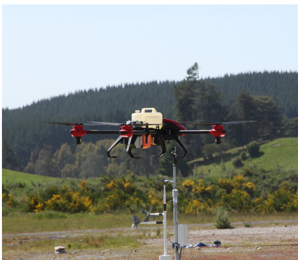
FIGURE 2: XAG P20 fitted with spinning disc atomisers under each rotor (Photo credit: Brian Richardson).
