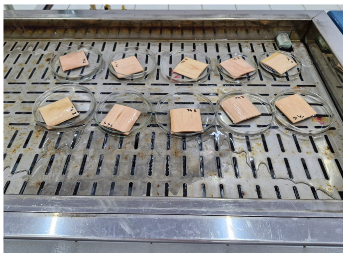
FIGURE 1: Bleaching of Eucalyptus grandis veneers in hydrogen peroxide solution
