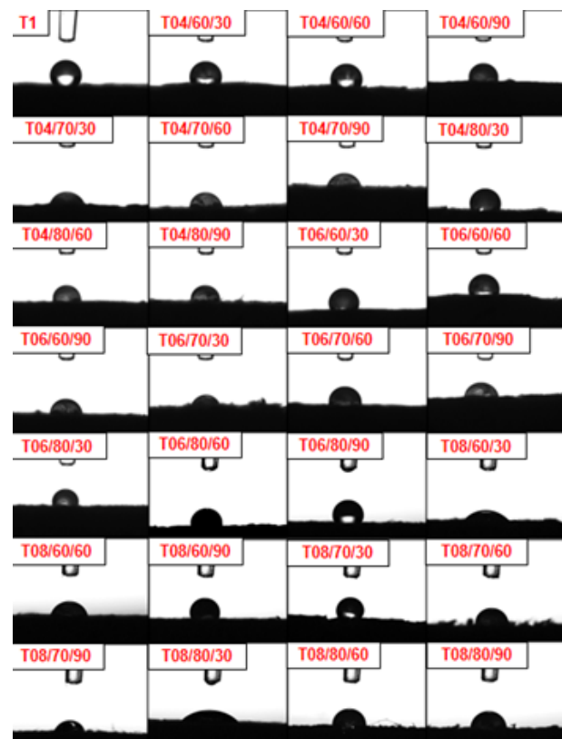
FIGURE 2: Contact angle between water droplets and the E. grandis veneers bleached with \text{H}_2\text{O}_2 under different conditions (pH/temperature/time).
